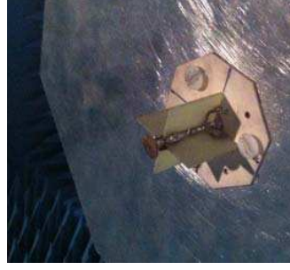
Figure 6. Prototype of the sensor A on a metallic plate of 300 mm in diameter.
