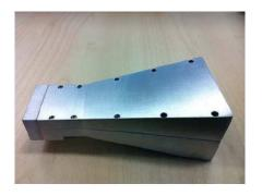
Figure 8. Prototype of the feed pyramidal horn antenna.
