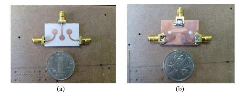
Figure 2. Photograph of the power divider. (a) Top layer. (b) Bottom layer.
