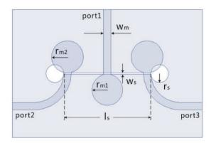
Figure 1. Configuration of the power divider.
