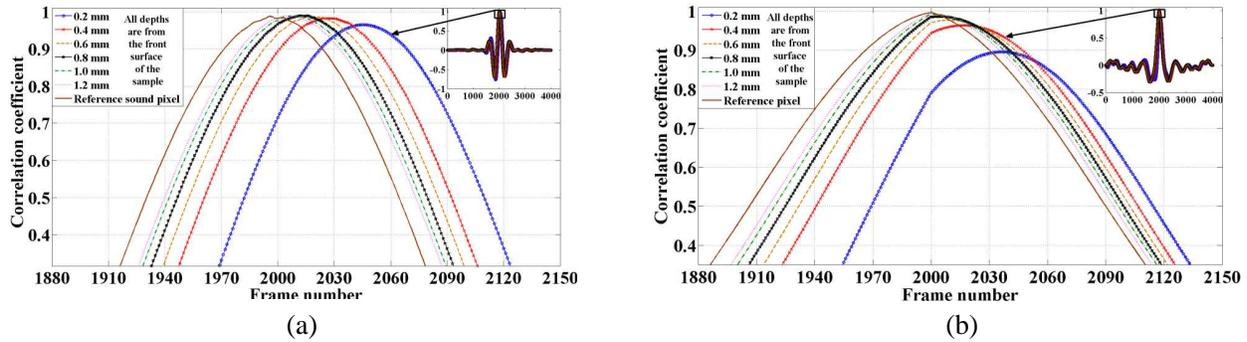
**Figure 4.** Obtained correlation profiles at various defect locations in the mild steel sample (inset shows compressed pulse). (a) Obtained correlation profiles for GLFMTWI. (b) Obtained correlation profiles for LFMTWI.
