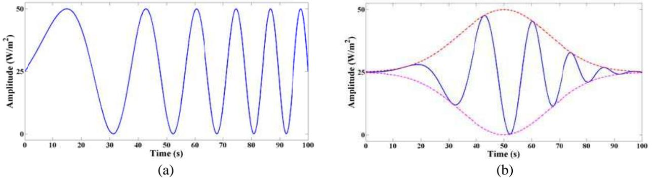
**Figure 1.** (a) Linear frequency modulated signal and (b) its Gaussian weighted form.
