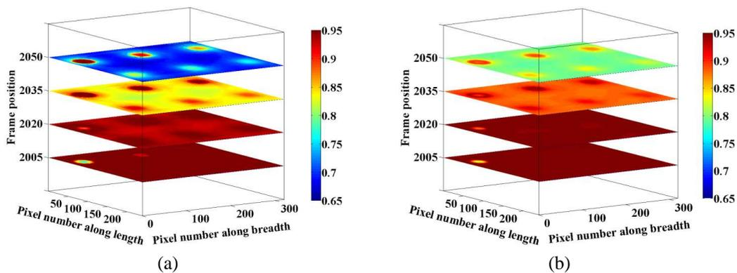
Figure 3. Depth scanning performance. (a) Depth scanning obtained from Gaussian weighted chirp LFMTWI. (b) Depth scanning obtained from LFMTWI.
