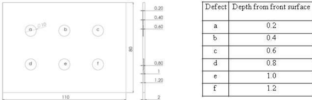
Figure 2. Top and cross-sectional view of simulated mild steel sample (all dimensions are in mm).
