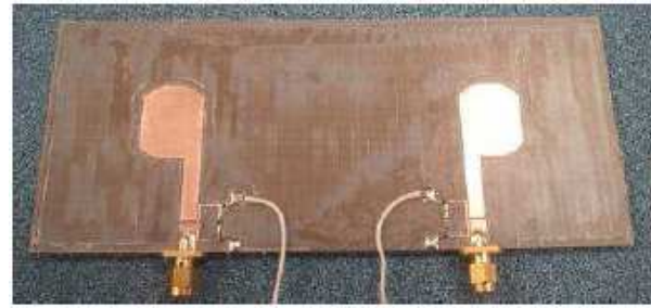
Figure 24. A fabricated prototype of the proposed polarization diversity tunable filter-antenna.
