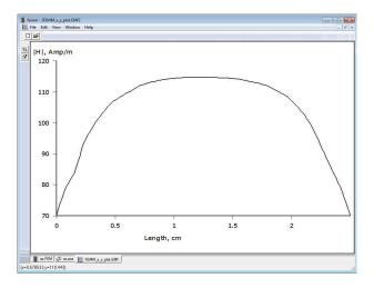
Figure 6. Axial homogeneity of the magnetic field obtained from FEMM.
