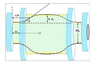
**Figure 2.** Combined representation of discrete step bobbin and shape modified bobbin. M is the field concentrated region for the discrete coil design. The profile of the shape modified bobbin, for the left half of its length, is defined by the generalized logistic function. The profile of the rest half is the mirror image of the former.  $\theta = \tan^{-1} B \frac{R_f - R_0}{4}$  for the shape modified bobbin.
