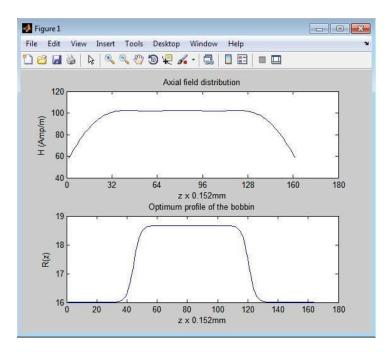
Figure 4. Axial field distribution and the optimum profile of the bobbin obtained by GA using MATLAB. The abcisa is in terms of the width (0.152 mm) of the wire (38 SWG). The values  $R_f = 8.28$  and C = 15.4 as obtained by GA optimization.
