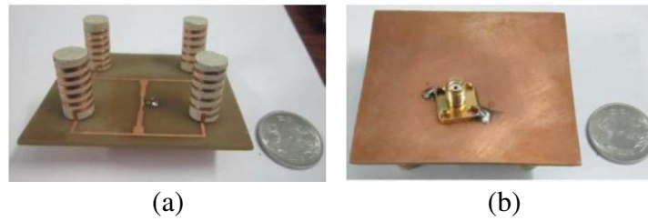
Figure 2. Photograph of fabricated antenna. (a) Top view. (b) Bottom view.
