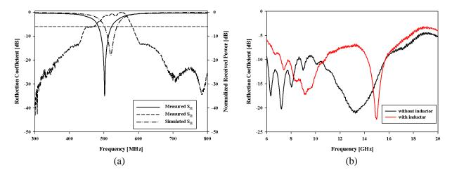
Figure 4. (a) Transmission and reflection characteristics of antenna. (b) Reflection coefficient of bowtie antenna with and without inductor, Bl = 11 mm, Fl = 8.4 mm, Sl = 4 mm, Sw = 3 mm, Sg = 0.2 mm, Iw = 0.3 mm, h = 1.6 mm, L = 11.1 mm, W = 12 mm.
