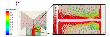
Figure 6. Surface current distribution at 503 MHz, Bl = 11 mm, Fl = 8.4 mm, Sl = 4 mm, Sw = 3 mm, Sg = 0.2 mm, Iw = 0.3 mm, h = 1.6 mm, L = 11.1 mm, W = 12 mm.
