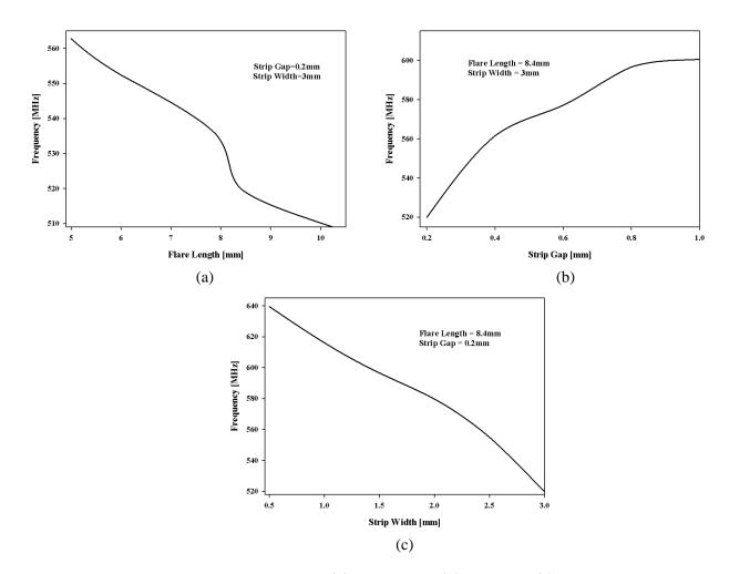
Figure 8. Resonant frequency variation with (a) flare length, (b) strip gap, (c) strip width, Bl = 11 mm, Sl = 4 mm, Iw = 0.3 mm, h = 1.6 mm, L = 11.1 mm, W = 12 mm.
