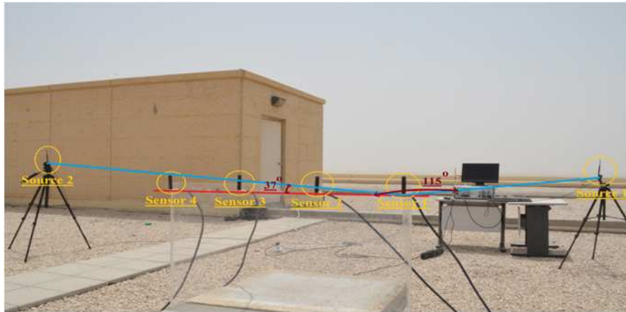
Figure 19. Experimental configuration of two RF sources placed at 37^\circ and 115^\circ from the array reference.
