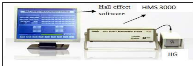
Figure 6. Hall effect measurement HMS 3000 setup.
