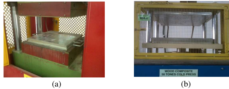
Figure 2. Wood plastic composite machine: (a) hot press machine, (b) cold press machine.
