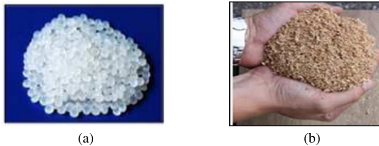
Figure 1. Wood plastic composite raw material: (a) PP crystalline, (b) Leucaena Leucocephala stems Sawdust filler.
