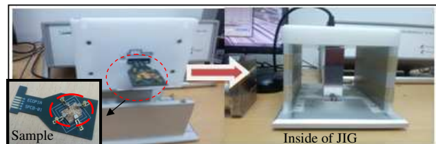
Figure 7. Sample PB board placement inside of jig.
