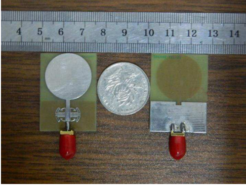
Figure 10. Photos of the fabricated prototypes for proposed antenna.
