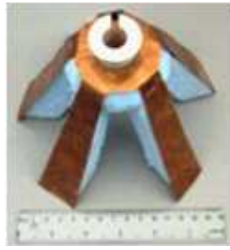
Figure 19. Configuration of inverted conical DRR with a skirt-shaped ground plane [100].
