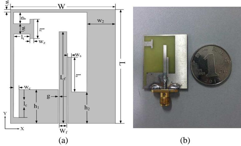
**Figure 1.** (a) Geometry of the proposed antenna. (b) Photograph of the manufactured antenna.
