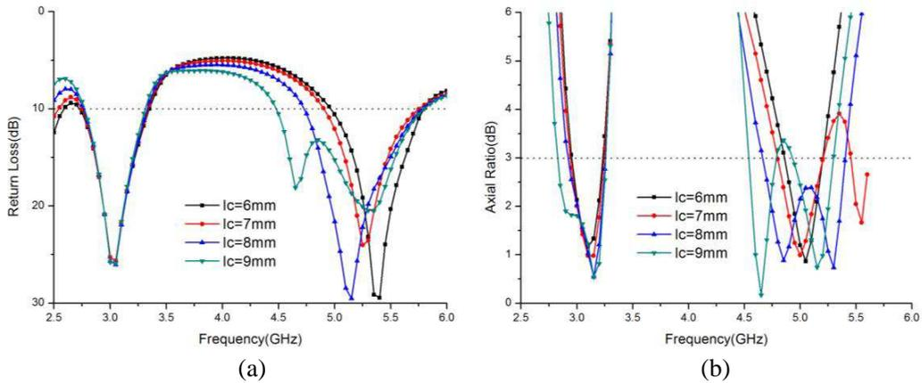
**Figure 4.** Simulated return loss and AR with different slit length ( $l_c$ ). (a) Return loss. (b) AR in the  $+z$  direction.
