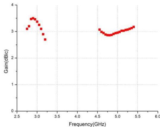
**Figure 9.** The measured peak gain versus frequency.
