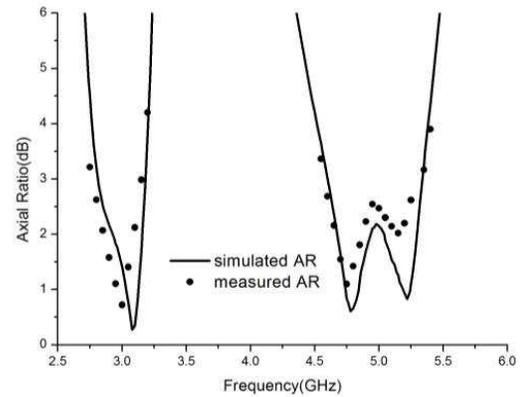
**Figure 7.** Simulated and measured axial ratio of the proposed antenna.
