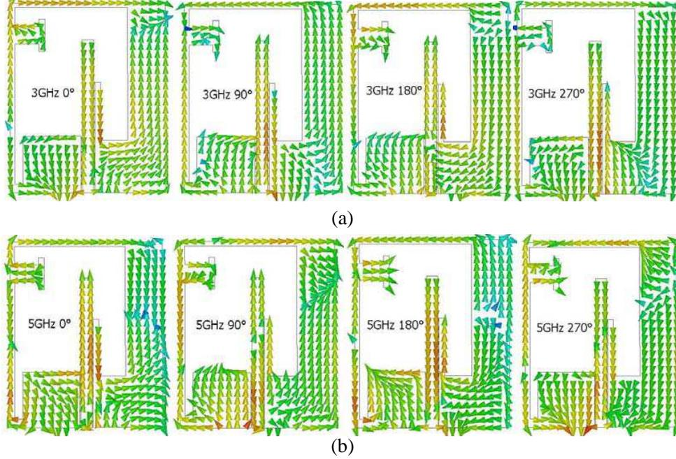
**Figure 5.** Surface current distributions of the proposed antenna in  $0^\circ$ ,  $90^\circ$ ,  $180^\circ$  and  $270^\circ$  phase. (a) 3 GHz. (b) 5 GHz.
