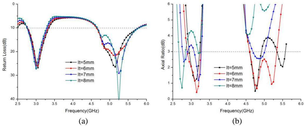
**Figure 3.** Simulated return loss and AR with different T-shaped strip length ( $l_t$ ). (a) Return loss. (b) AR in the  $+z$  direction.
