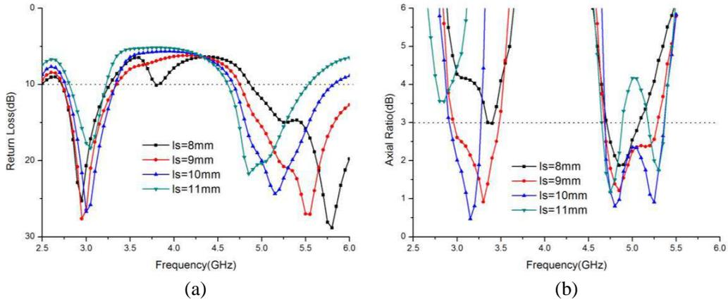
**Figure 2.** Simulated return loss and AR with different vertical stub length ( $l_s$ ). (a) Return loss. (b) AR in the  $+z$  direction.
