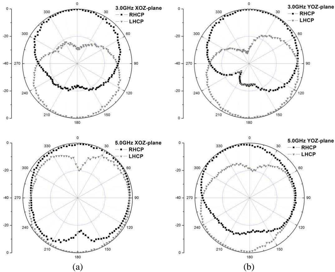
**Figure 8.** Measured radiation patterns of the proposed antenna at 3 GHz and 5 GHz. (a)  $XOZ$ -plane. (b)  $YOZ$ -plane.
