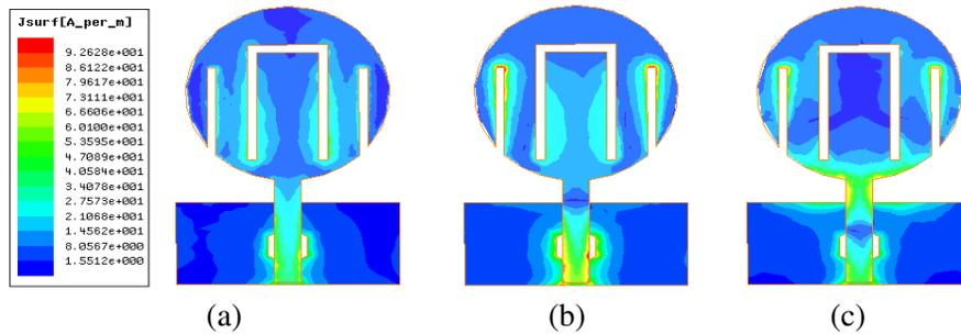
**Figure 6.** Current distribution of the proposed antenna at (a) 2.45 GHz. (b) 3.5 GHz. (c) 5.65 GHz.
