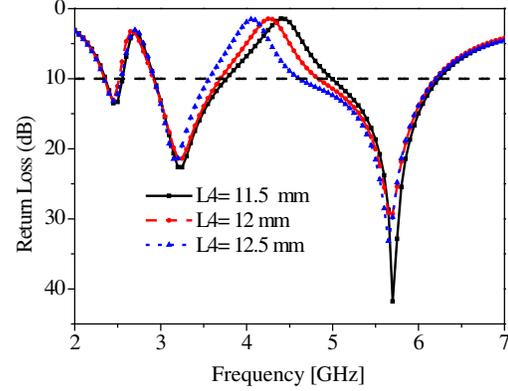
**Figure 2.** Simulated return loss of the proposed antenna for various length of  $L_4$ .
