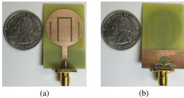
**Figure 5.** Photograph of the proposed antenna. (a) Top view; (b) Bottom view.
