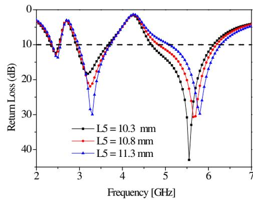
**Figure 4.** Simulated return loss of the proposed antenna for various length of  $L_5$ .
