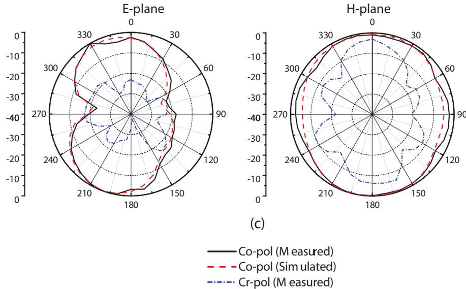
**Figure 8.** Normalized measured co- and cross polarization radiation pattern at (a) 2.45 GHz, (b) 3.5 GHz, (c) 5.5 GHz.
