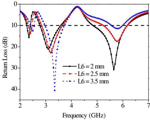
**Figure 3.** Simulated return loss of the proposed antenna for various length of  $L_6$ .
