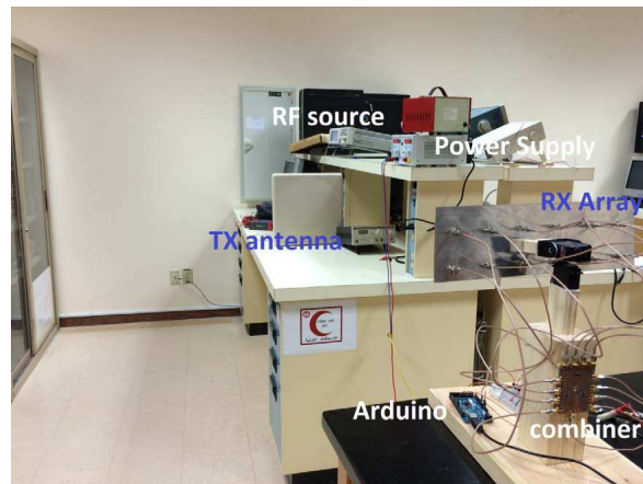
Figure 13. Experimental setup showing the various components of the system.
