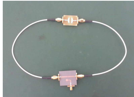
Figure 17. Photo of the proposed antenna connected with the out-of-phase power divider.
