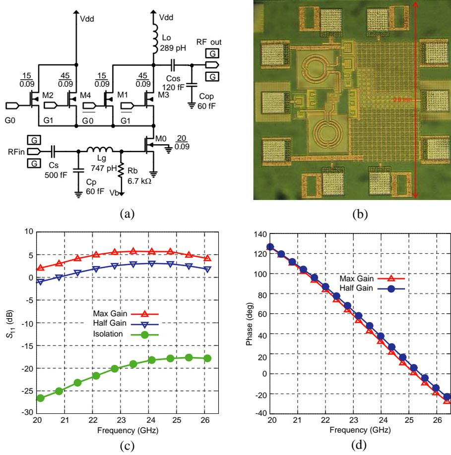
**Figure 8.** VGA schematic, die photo, simulated and measured results. (a) Schematic of VGA. (b) Die photo of VGA. (c) VGA measured gain for programmed states. (d) VGA measured phase for programmed states.
