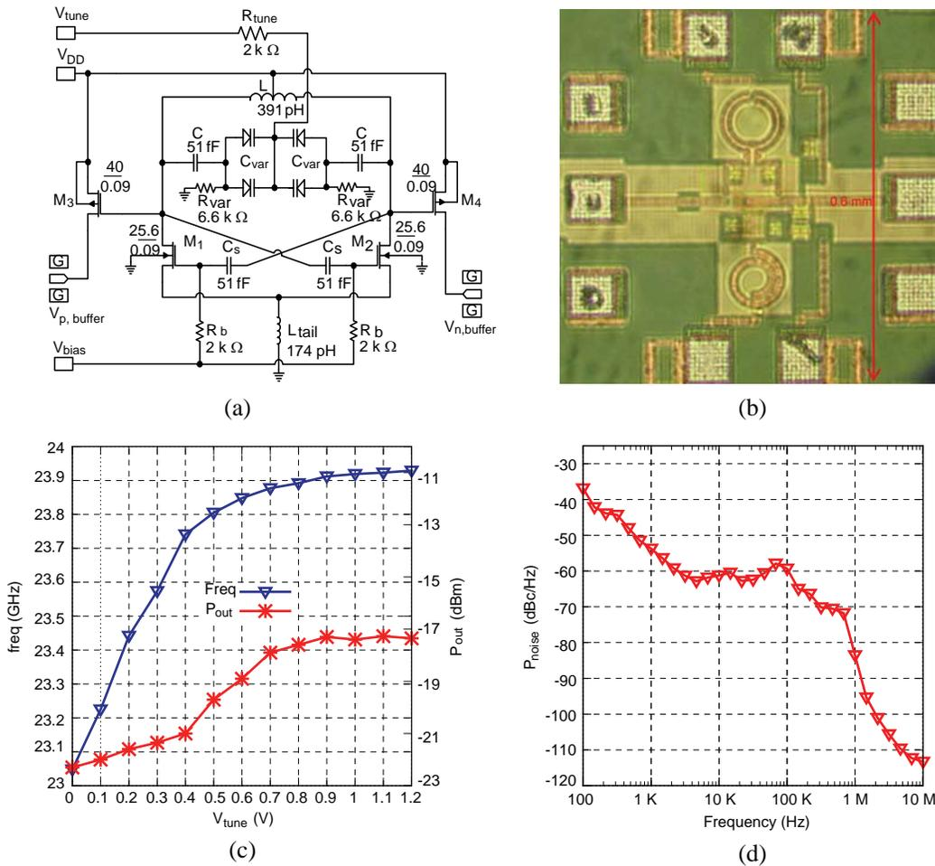
**Figure 10.** VCO schematic, die photo and measured results. (a) Cross-coupled VCO schematic. (b) Die photo of VCO. (c) VCO tuning range and output power without losses of cables and connectors. (d) Locked phase noise of the designed VCO with commercial PLL chip.
