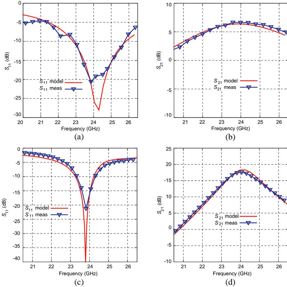
**Figure 7.** LNA parasitic models and their measurement results. (a) Measured and simulated  $S_{11}$  of 1-stage LNA: parasitic modelled. (b) Measured and simulated  $S_{21}$  of 1-stage LNA: parasitic modelled. (c) Measured and simulated  $S_{11}$  of 3-stage LNA: parasitic modelled. (d) Measured and simulated  $S_{21}$  of 3-stage LNA: parasitic modelled.
