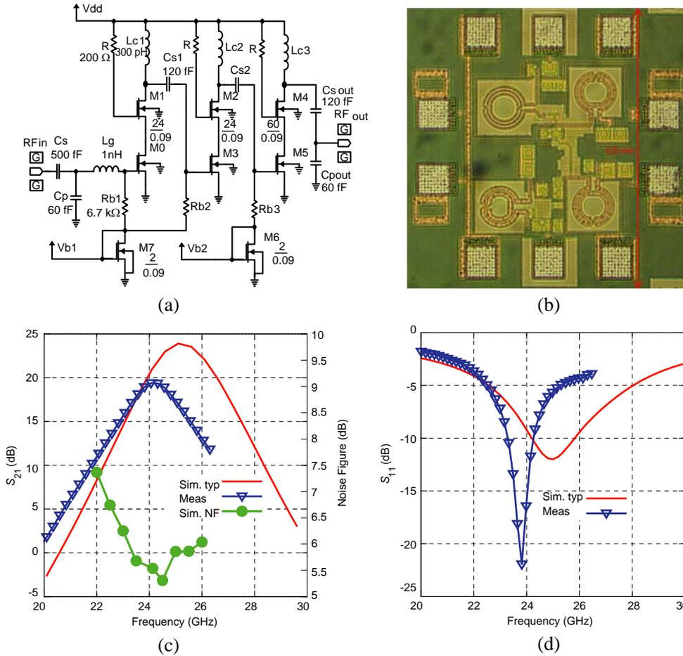
**Figure 5.** Three-stage LNA schematic, die photo, simulated and measured  $S$ -parameters. (a) Schematic of 3-stage LNA. (b) Die photo of 3-stage LNA. (c) Simulated and measured LNA gain. (d) Simulated and measured LNA return loss.
