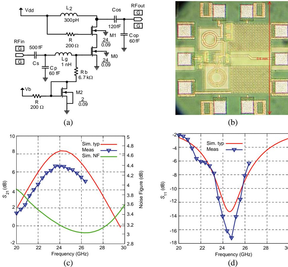
**Figure 4.** Single-stage LNA schematic, die photo, simulated and measured  $S$ -parameters. (a) Schematic of 1-stage LNA. (b) Die photo of 1-stage LNA. (c) Simulated and measured LNA gain. (d) Simulated and measured LNA return loss.
