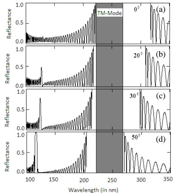
**Figure 12.** TM-reflectance spectra of a photonic quantum well structure  $(EF)^{30}$  for incidence angles (a)  $0^\circ$ , (b)  $20^\circ$ , (c)  $30^\circ$ , and (d)  $50^\circ$  having thicknesses  $d_E = 46.7$  nm and  $d_F = 26.7$  nm.
