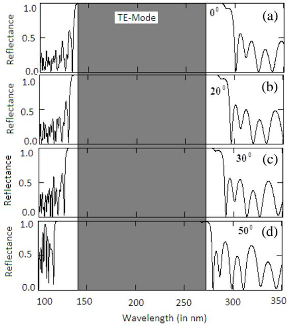
**Figure 5.** TE-reflectance spectra of a photonic quantum well structure  $(AB)^{10}/(CD)^{10}/(EF)^{10}$  for incidence angles (a)  $0^\circ$ , (b)  $20^\circ$ , (c)  $30^\circ$ , and (d)  $50^\circ$  having thicknesses  $d_A = 28.8$  nm,  $d_B = 16.4$  nm,  $d_C = 36$  nm,  $d_D = 20.5$  nm,  $d_E = 43.2$  nm, and  $d_F = 24.6$  nm, respectively.
