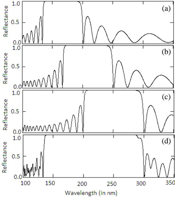
**Figure 2.** Reflectance spectra of a photonic quantum well structure at normal incidence for (a)  $(AB)^{10}$ , (b)  $(CD)^{10}$ , (c)  $(EF)^{10}$ , and (d)  $(AB)^{10}/(CD)^{10}/(EF)^{10}$  having thicknesses  $d_A = 28.8$  nm,  $d_B = 16.4$  nm,  $d_C = 36$  nm,  $d_D = 20.5$  nm,  $d_E = 43.2$  nm, and  $d_F = 24.6$  nm, respectively.
