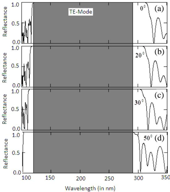
**Figure 9.** TE-reflectance spectra of a photonic quantum well structure  $(AB)^{10}/(CD)^{10}/(EF)^{10}$  for incidence angles (a)  $0^\circ$ , (b)  $20^\circ$ , (c)  $30^\circ$ , and (d)  $50^\circ$  having thicknesses  $d_A = 25.2\text{ nm}$ ,  $d_B = 14.3\text{ nm}$ ,  $d_C = 36\text{ nm}$ ,  $d_D = 20.5\text{ nm}$ ,  $d_E = 46.7\text{ nm}$ , and  $d_F = 26.7\text{ nm}$ , respectively.
