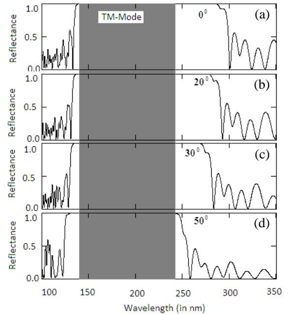
**Figure 6.** TM-reflectance spectra of a photonic quantum well structure  $(AB)^{10}/(CD)^{10}/(EF)^{10}$  for incidence angles (a)  $0^\circ$ , (b)  $20^\circ$ , (c)  $30^\circ$ , and (d)  $50^\circ$  having thicknesses  $d_A = 28.8$  nm,  $d_B = 16.4$  nm,  $d_C = 36$  nm,  $d_D = 20.5$  nm,  $d_E = 43.2$  nm, and  $d_F = 24.6$  nm, respectively.
