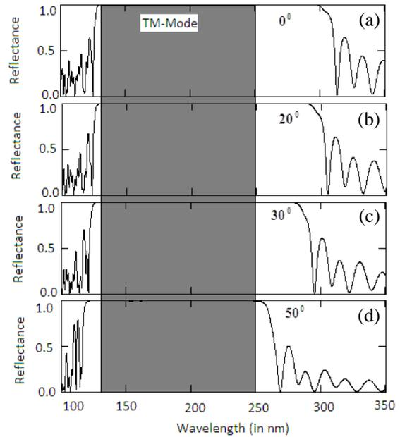
**Figure 8.** TM-reflectance spectra of a photonic quantum well structure  $(AB)^{10}/(CD)^{10}/(EF)^{10}$  for incidence angles (a)  $0^\circ$ , (b)  $20^\circ$ , (c)  $30^\circ$ , and (d)  $50^\circ$  having thicknesses  $d_A = 27$  nm,  $d_B = 15.4$  nm,  $d_C = 36$  nm,  $d_D = 20.5$  nm,  $d_E = 45$  nm, and  $d_F = 25.6$  nm, respectively.
