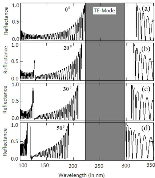
**Figure 11.** TE-reflectance spectra of a photonic quantum well structure  $(EF)^{30}$  for incidence angles (a)  $0^\circ$ , (b)  $20^\circ$ , (c)  $30^\circ$ , and (d)  $50^\circ$  having thicknesses  $d_E = 46.7$  nm and  $d_F = 26.7$  nm.
