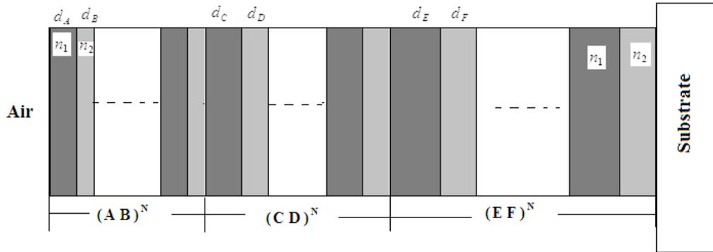
**Figure 1.** Schematic representation of one-dimensional multi quantum well photonic crystal structure.
