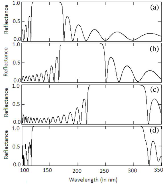
**Figure 4.** Reflectance spectra of a photonic quantum well structure for (a)  $(AB)^{10}$ , (b)  $(CD)^{10}$ , (c)  $(EF)^{10}$ , and (d)  $(AB)^{10}/(CD)^{10}/(EF)^{10}$  and for thicknesses  $d_A = 25.2$  nm,  $d_B = 14.3$  nm,  $d_C = 36$  nm,  $d_D = 20.5$  nm,  $d_E = 46.7$  nm, and  $d_F = 26.7$  nm, respectively.
