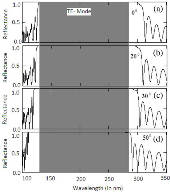
**Figure 7.** TE-reflectance spectra of a photonic quantum well structure  $(AB)^{10}/(CD)^{10}/(EF)^{10}$  for incidence angles (a)  $0^\circ$ , (b)  $20^\circ$ , (c)  $30^\circ$ , and (d)  $50^\circ$  having thicknesses  $d_A = 27$  nm,  $d_B = 15.4$  nm,  $d_C = 36$  nm,  $d_D = 20.5$  nm,  $d_E = 45$  nm, and  $d_F = 25.6$  nm, respectively.
