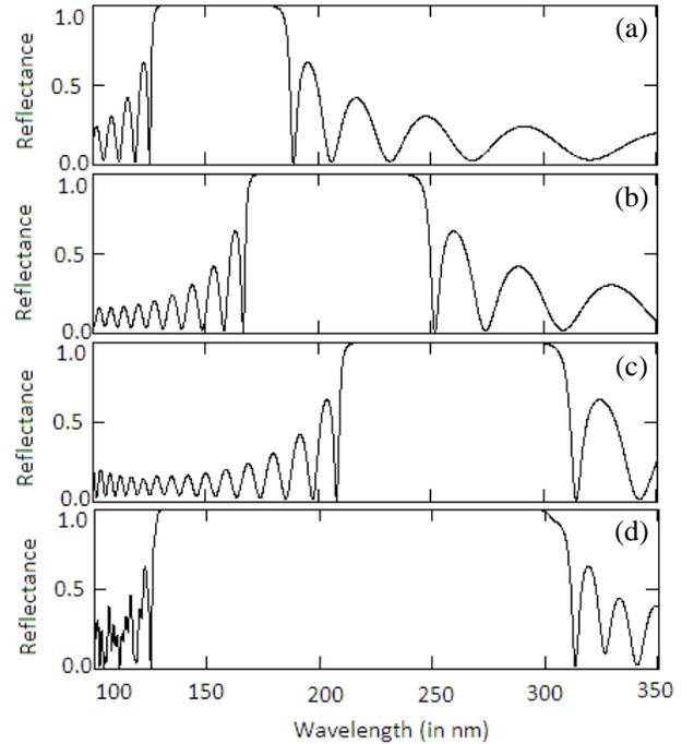
**Figure 3.** Reflectance spectra of a photonic quantum well structure at normal incidence for (a)  $(AB)^{10}$ , (b)  $(CD)^{10}$ , (c)  $(EF)^{10}$  and (d)  $(AB)^{10}/(CD)^{10}/(EF)^{10}$  having thicknesses  $d_A = 27$  nm,  $d_B = 15.4$  nm,  $d_C = 36$  nm,  $d_D = 20.5$  nm,  $d_E = 45$  nm, and  $d_F = 25.6$  nm, respectively.
