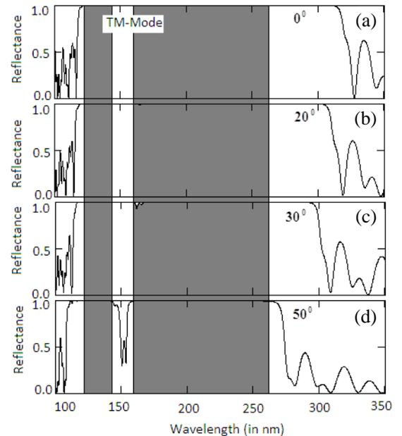
**Figure 10.** TM-reflectance spectra of a photonic quantum well structure  $(AB)^{10}/(CD)^{10}/(EF)^{10}$  for incidence angles (a)  $0^\circ$ , (b)  $20^\circ$ , (c)  $30^\circ$ , and (d)  $50^\circ$  having thicknesses  $d_A = 25.2\text{ nm}$ ,  $d_B = 14.3\text{ nm}$ ,  $d_C = 36\text{ nm}$ ,  $d_D = 20.5\text{ nm}$ ,  $d_E = 46.7\text{ nm}$ , and  $d_F = 26.7\text{ nm}$ , respectively.
