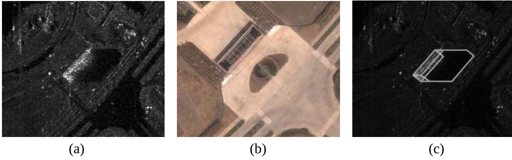
Figure 13. Airborne SAR data experiment. (a) Airborne SAR image chip. (b) Optical image (©Google Earth). (c) Overlaid with the predicted building geometrical structure.
