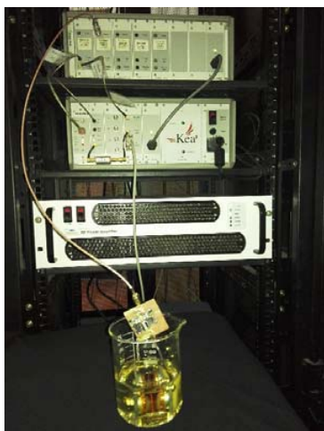
Figure 5. A photo of the measurement system, the sensor was immersed into the turbine oil.
