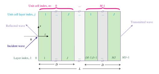
Figure 1. Geometry under consideration consisting of a one-dimensional periodic layered medium bounded by two semi-infinite half spaces and composed of M repeated unit cells, each consisting of Jlayers. The medium is excited from one half-space by an incident plane inclined at an arbitrary angle  $\theta$  in the xz plane.
