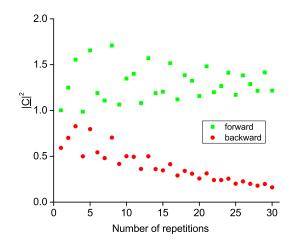
Figure 3. Forward and backward components of the weighting matrix  $|\underline{C}|^2$  versus the number of repetitions. Here, we have assumed a metal-dielectric bi-layer system with a unit cell made from a 30-nm-thick Ag layer and 30-nm-thick TiO<sub>2</sub> layer, assuming a normally incident TM-polarized wave with a free-space wavelength of  $\lambda_0 = 365$  nm.
