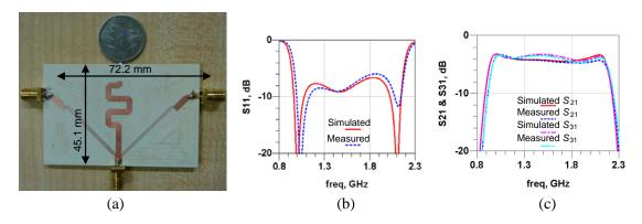
**Figure 8.** (a) Photograph of the designed T-junction divider. (b) Simulated/measured Return loss of port 1. (c) Simulated/measured transmissions.
