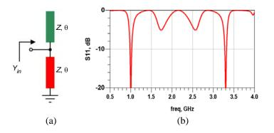
**Figure 9.** (a) A dual-band complex impedance using parallel combinations of open and short stubs to fine-tune out-of-the-band performance. (b) Simulated Return loss for the case4 of Table 1 showing better out-of-the-band performance.
