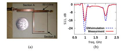
**Figure 6.** (a) The manufactured prototype in our lab. This is a configuration-I type matching network. (b) The measurement result as compared to the EM-simulation result.
