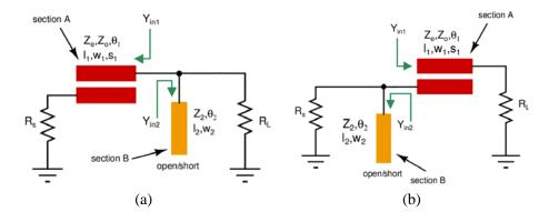
**Figure 1.** Proposed dual-band matching networks. (a) Configuration-I: stub on the load side. (b) Configuration-II: stub on the source side.
