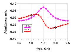
Figure 3. Variation of the real and imaginary parts of  $Y_{in1}$ . Re(·) returns the real part of a complex number whereas Im(·) returns the imaginary part.
