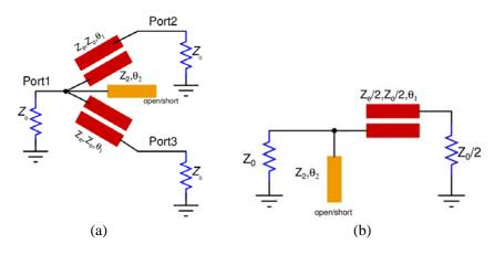
**Figure 7.** (a) A dual-band T-junction power divider. (b) Equivalent circuit of the divider looking into the port 1.
