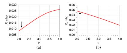
**Figure 2.** Variation of P and Q ( $@f_1$ ) with  $\rho$  in the above example. (a) Plot of P: arrow indicates the value of  $\rho$  (= 2.1332) where the value of P = 0.01 mho. (b) Plot of Q: arrow indicates the value of Q corresponding to  $\rho = 2.1332$ .
