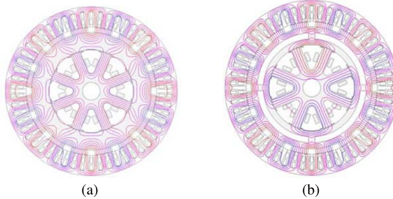
Figure 6. Magnetic field distribution diagram. (a) Solid rotor. (b) The distributed hollow rotor.
