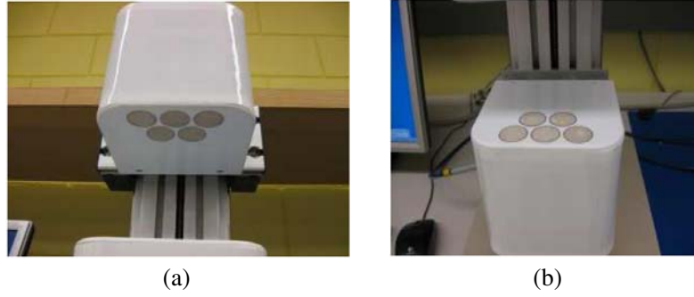
Figure 7. Setup of Nahanni transmission measurement system. (a) View of the upper array consisting of five Nahanni sensors, and (b) view of the lower array consisting of five Nahanni sensors. In (a) and (b), the brown circle on the upper and the lower arrays indicates the aperture of Nahanni sensor.
