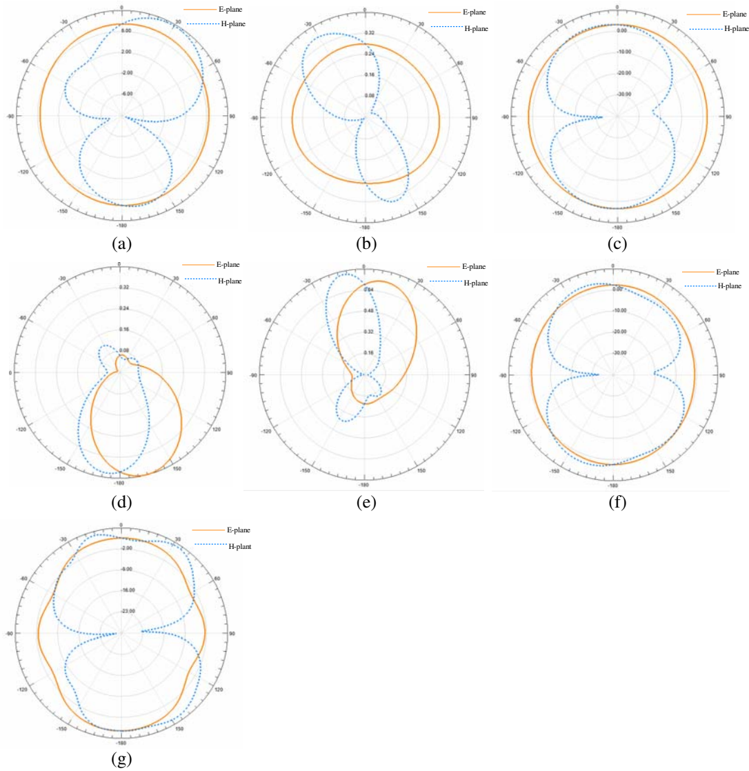
Figure 5. Measured radiation pattern of the UWB planar monopole antenna: (a) 2.5 GHz, (b) 4.0 GHz, (c) 5.0 GHz, (d) 5.2 GHz, (e) 6.8 GHz, (f) 7.5 GHz, (g) 10.0 GHz.
