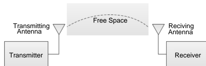
Figure 1. Functional blocks of a typical Wireless Power Transfer (WPT) system.
