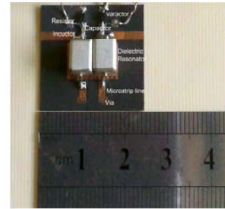
Figure 12. Photo of the fabricated filter.
