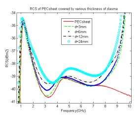
**Figure 10.** RCS of Perfect Electric Conductor (PEC) when it is not covered by plasma layer and when it is covered by plasma layer of different thickness.
