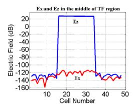
**Figure 5.** Power isolation on TF/SF interface for DPW method.
