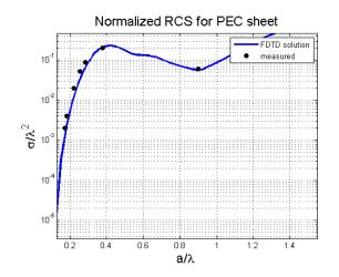
Figure 7. Comparison between measured and simulated RCS of PEC at different wavelengths.
