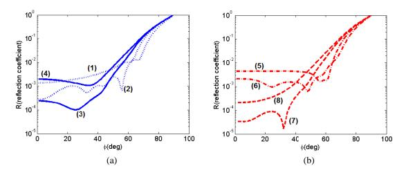
Figure 15. Reflection coefficient from conductive sheet covered by inhomogeneous profile (a) TE mode (solid) polynomial and (dotted) exponential and (b) TM mode (dash-dash) polynomial and (dash-point) exponential. For all graphs  $k_{fd} = n_{fd} = 1$ ,  $k_{f0} = 0$ ,  $n_{f0} = 1$ ,  $d_f = 0.09$  m, (1, 3, 5 and 7) a = 3.5 (2, 4, 6 and 8) a = 5.
