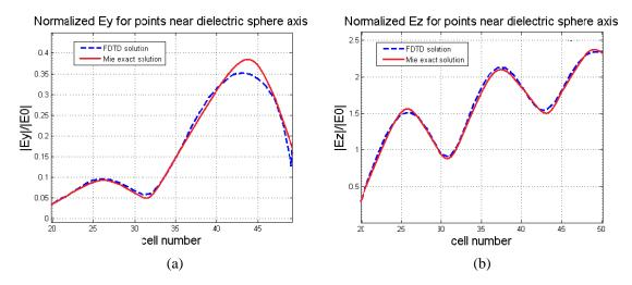
**Figure 6.** Normalized electric fields  $(E_z \text{ and } E_x)$  on the axis of dielectric sphere. (a)  $\frac{E_y}{E_0}$ . (b)  $\frac{E_z}{E_0}$ .
