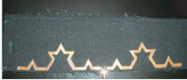
Figure 6. Fabricated photograph of Koch fractal antenna on jeans cloth.
