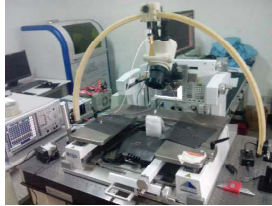
Figure 6. Photograph of the antenna measurement system in lab.
