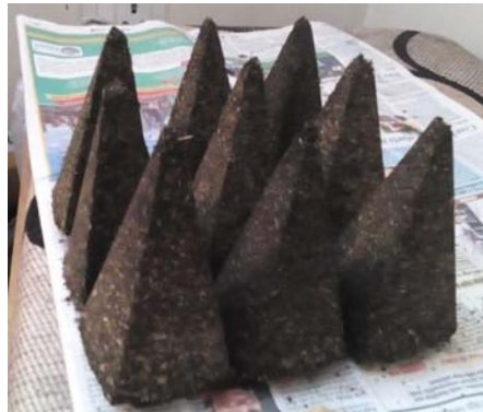
Figure 4. 3 \times 3 pyramidal microwave absorber.
