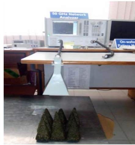
Figure 7. Set up for testing 3 \times 3 array by RCS method [15].
