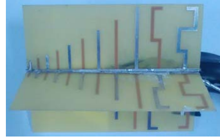
Figure 3. Photograph of the fabricated dual-polarized meander line log-periodic antenna.
