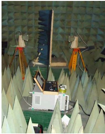
Figure 7. Experiment setup for measuring insertion loss of ESS.
