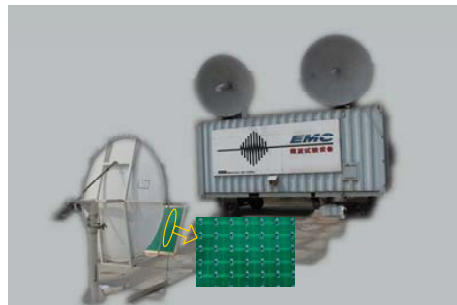
Figure 9. Measurement setup for shielding effectiveness of ESS under irradiating by HPM.
