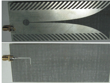
Figure 2. Fabricated samples of the Vivaldi antenna with ESCE.
