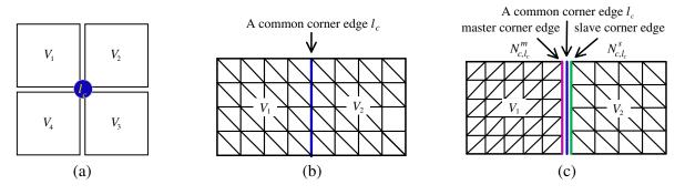
Figure 2. Conformal and non-conformal mesh case for a common corner edge.
