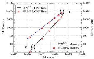
**Figure 4.** CPU time and memory cost as a function of unknowns for factorizing  $[\tilde{K}_{cc}]$ .
