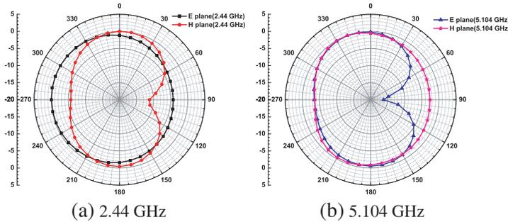
Figure 14. Simulated  $E$  field and  $H$  field radiation patterns of SISO ( $x$ - $y$  plane).
