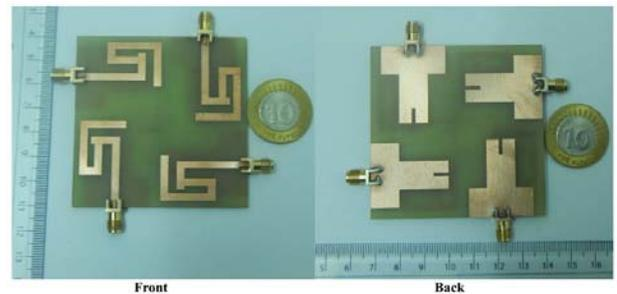
**Figure 2.** Fabricated  $2 \times 2$  MIMO antenna.
