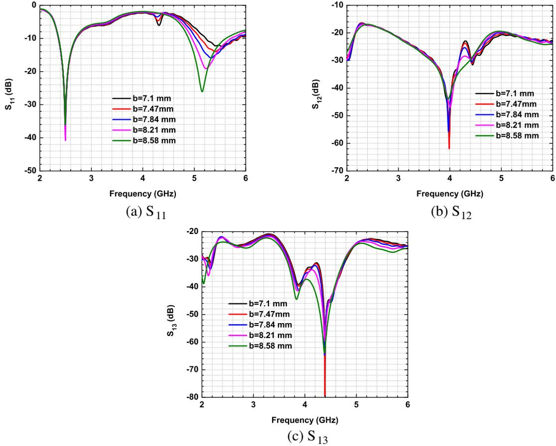
Figure 10. Effect of arm  $b$  on  $S$  parameters.
