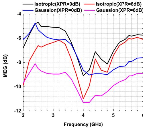
**Figure 13.** MEG comparisons between isotropic and gaussian mediums.
