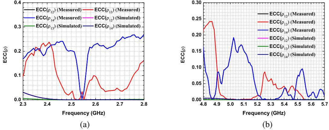
**Figure 12.** ECC of proposed  $2 \times 2$  MIMO antenna. (a) ECC in lower band. (b) ECC in higher band.
