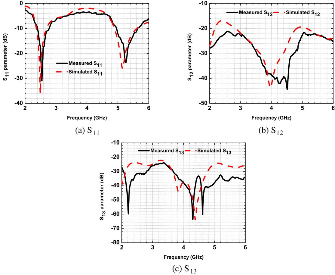
**Figure 4.**  $S$  parameters of proposed  $2 \times 2$  MIMO antenna.
