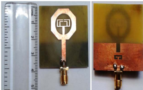
Figure 10. Image of the fabricated split ring loaded triple band antenna ‘c’: (a) top view; (b) bottom view.
