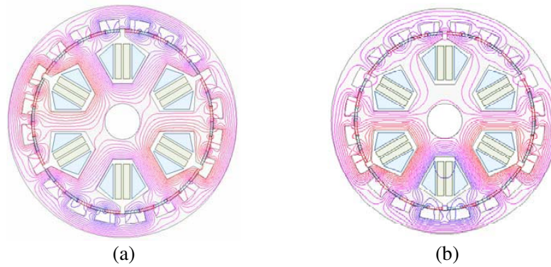
Figure 7. No-load magnetic field distributions of the HE-SPMVM. (a) PMs excitation only. (b) PMs and field winding excitations.
