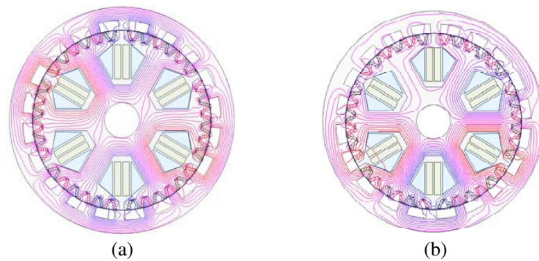
Figure 8. No-load magnetic field distributions of the HE-VIPMVM. (a) PMs excitation only. (b) PMs and field winding excitations.
