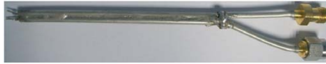
Figure 6. Differential probe used to characterize the antennas.
