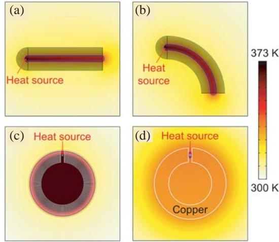
**Figure 3.** (Color Online) Temperature distributions of flexible thermal hoses made of copper and expanded polystyrene in bilayer configurations. (a) A straight thermal hose cascaded with a semi-circular super-insulating shell. (b) A curved thermal hose cascaded with a semi-circular super-insulating shell. (c) A SRS hose. (d) The reference structure composed of bare copper. Isothermal lines are also represented with blue color in the panel.
