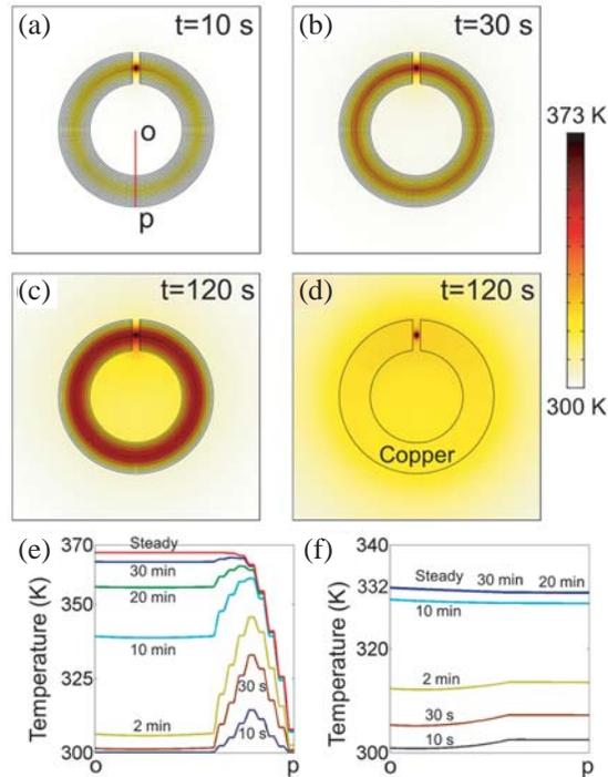
**Figure 4.** (Color Online) Transient temperature distributions of the SRS hose in Fig. 3(c) at different times (a)  $t = 10$ , (b)  $t = 30$ , (c)  $t = 120$  s. (d) Temperature distribution of the reference structure at  $t = 120$  s. (e) Thermal profile of the SRS hose in (a) along the observation line “op” at different times. (f) Thermal profile of the reference structure in (d) along observation line “op” at different times.
