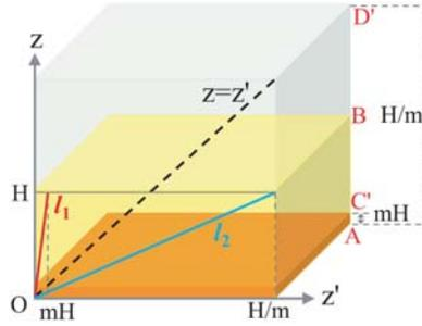
**Figure 1.** (Color Online) Schematic illustration of coordinate transformation in the design of thermal super-transferring and super-insulating slabs, where the former is generated by stretching  $AC'$  into  $AB$ , and the latter is generated by compressing  $AD'$  into  $AB$ , respectively.
