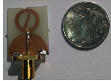
Figure 4. Prototype of the designed antenna.
