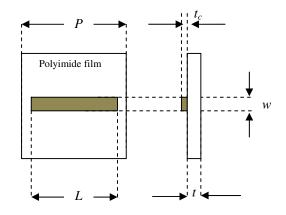
Figure 1. The unit cell of the dipole FSS.
