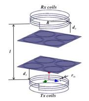
Figure 4. WPT system with MM slabs.
