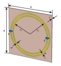
**Figure 2.** Schematic diagram of unit cell of CLSRRs.
