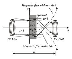
Figure 1. System configuration for the analysis of divergent field focus effect through MM slab.
