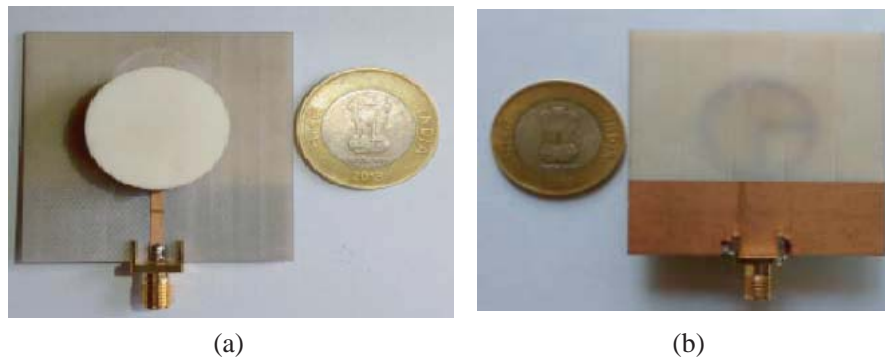
Figure 2. Archetype of proposed antenna Structure. (a) Top view. (b) Bottom view.
