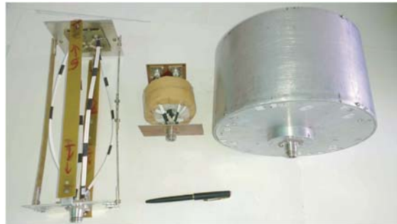
Figure 4. Fabricated 4-way power dividers — Straight (left) and coiled (centre). Also shown is 7-way enclosed coiled power divider (right) for size comparison.
