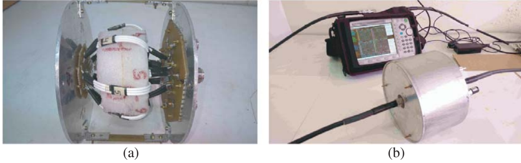
Figure 3. Fabricated 7-way power divider — open and enclosed. (a) 7-way power divider assembly (side open). (b) 7-way power divider (enclosed).
