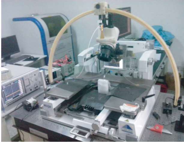
Figure 5. Overview of the antenna measurement system in lab.
