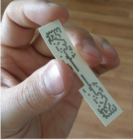
Figure 4. A fabricated pixel antenna for measurements. The antenna is produced via low-cost inkjet printing using standard printers.
