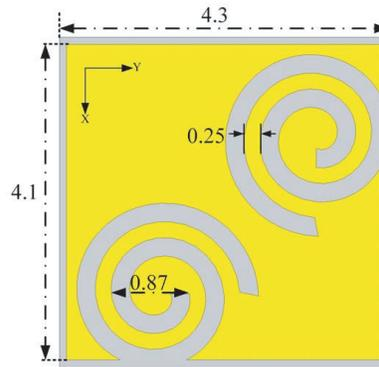
**Figure 1.** Geometry of EBG (unit in mm).
