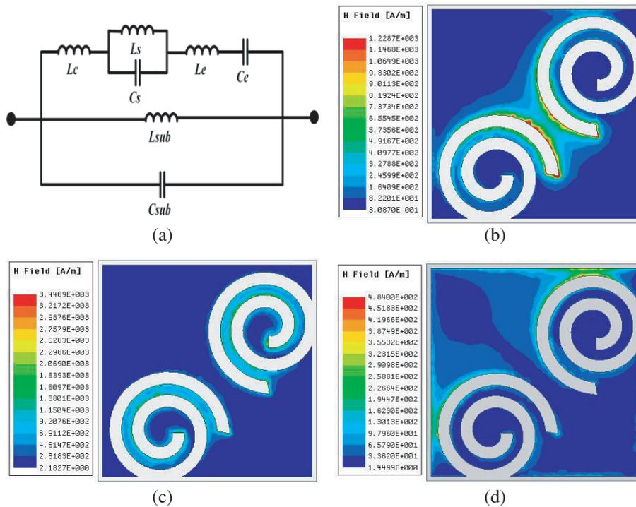
**Figure 2.** Equivalent model and magnetic field distribution of EBG irradiated by TM-polarized incident wave in normal direction. (a) Equivalent model of EBG. (b) Magnetic field distribution at 8.8 GHz. (c) Magnetic field distribution at 12 GHz. (d) Magnetic field distribution at 15.8 GHz.
