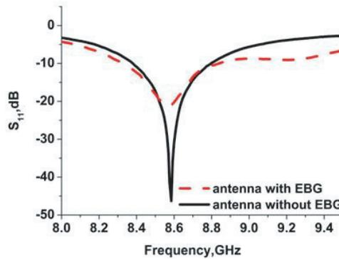
Figure 7. Measured  $S$ -parameter of antenna 1 with/without EBG.
