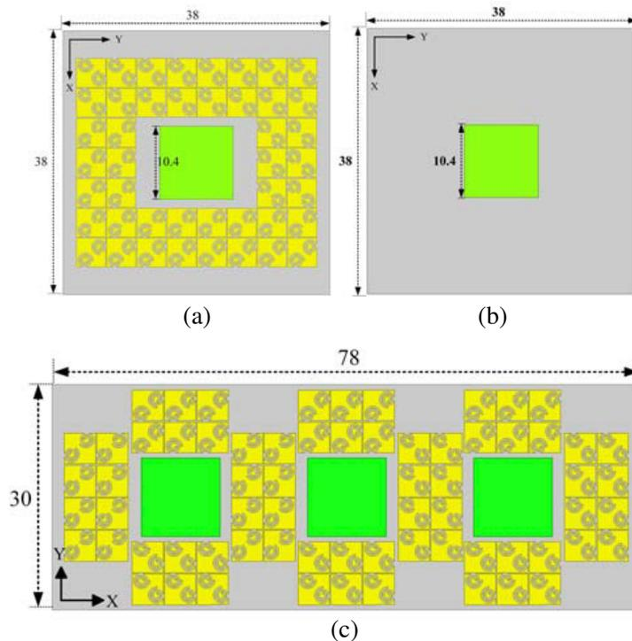
**Figure 4.** Geometry of antenna with/without EBG (unit in mm, antenna 1, 8.6 GHz). (a) Antenna unit with EBG. (b) Without EBG. (c) Antenna array with EBG.
