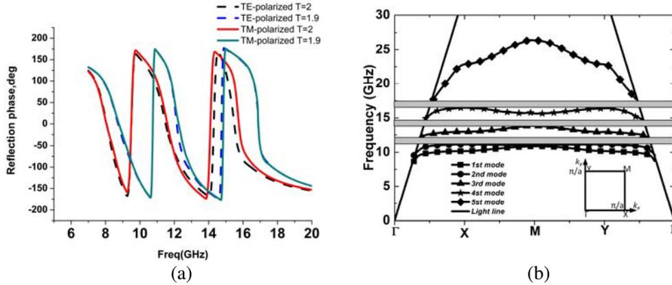
**Figure 3.** Reflection band-gaps and surface wave band-gaps of EBG structure. (a) Reflection band-gaps. (b) Dispersion diagram.
