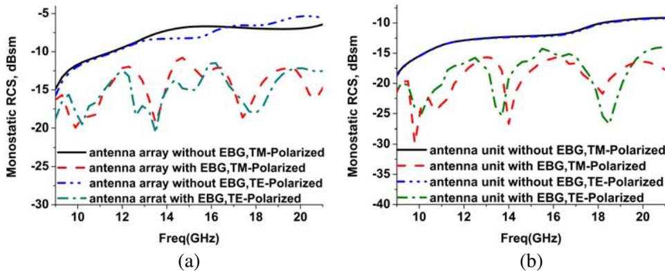
Figure 8. Monostatic RCS at normal incident waves. (a) Antenna 1 array. (b) Antenna 1 unit.
