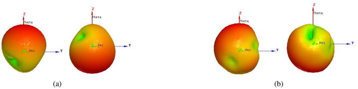
Figure 7. 3D radiation patterns at LHCP (left) and RHCP (right) planes at: (a) 5 GHz, (b) 8 GHz.
