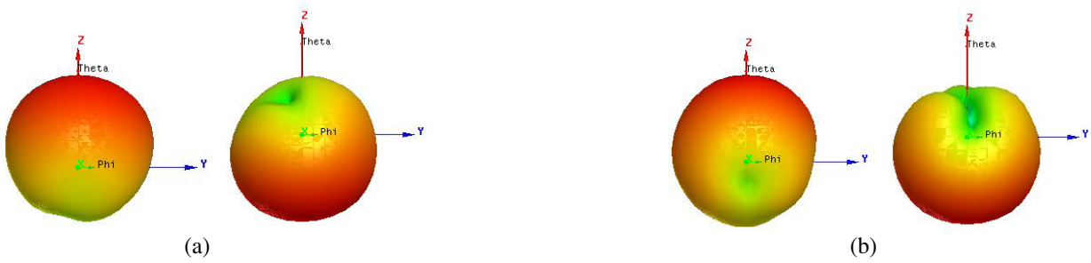
Figure 6. 3D radiation patterns at LHCP (left) and RHCP (right) planes at: (a) 6 GHz, (b) 7 GHz.
