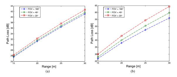
Figure 5. Curve of path loss for different link ranges. (a) Coastal water. (b) Harbor water.
