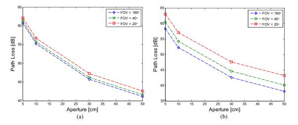
**Figure 6.** Curve of path loss for different apertures. (a) Coastal water (L = 30 m). (b) Harbor water (L = 9 m).
